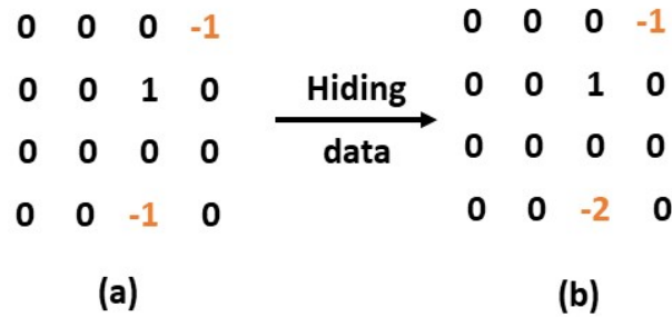
Fig. 4: The QDCT coefficients: (a) before and (b) after the embedding operation
