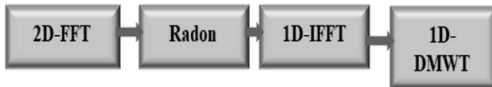
Figure 2: Iris recognition system using combination methods.
