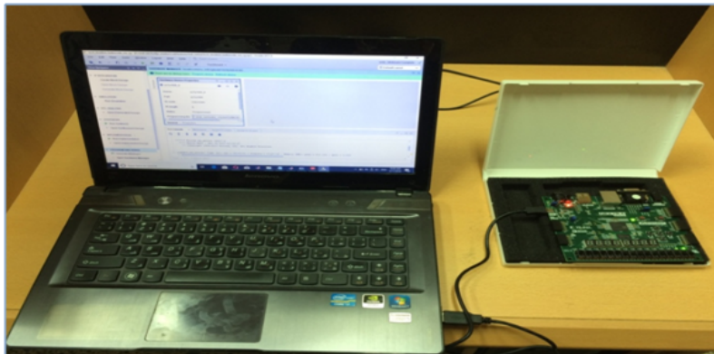
Figure 12: Real time implementation of turbo encoder using artix- 7 device
