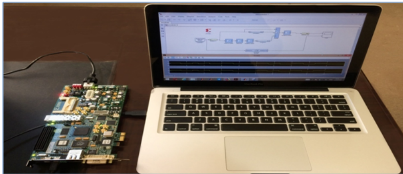
Figure 11: Real time implementation of turbo encoder using spartan- 6 device
